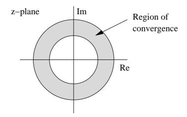
In specific cases the inner radius of this ring may include the origin, and the outer radius may extend to infinity. If the ROC includes the unit circle |z|=1, then the Fourier transform will converge.
