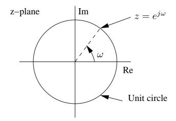
The inherent periodicity in frequency of the Fourier transform is captured naturally under this interpretation.
