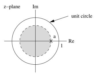
Note that the expression for the z-transform (and the pole zero plot) is exactly the same as for the right-handed exponential sequence — *only the region of convergence is different*. Specifying the ROC is therefore critical when dealing with the z-transform.
