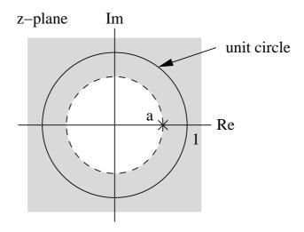
The Fourier transform of x[n] only exists if the ROC includes the unit circle, which requires that |a| < 1. On the other hand, if |a| > 1 then the ROC does not include the unit circle, and the Fourier transform does not exist. This is consistent with the fact that for these values of a the sequence  $a^n u[n]$  is exponentially growing, and the sum therefore does not converge.
