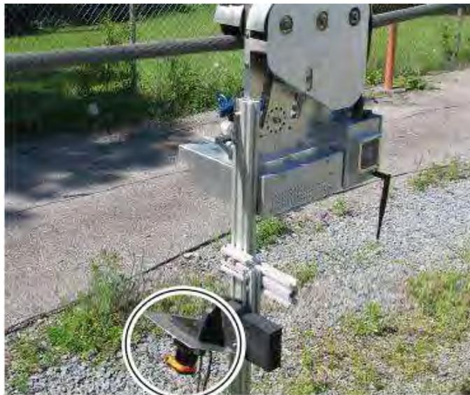
FIGURE 2.3: An older robot by Hydro-Québec, the LineROver, with a mounted UTM-30LX laser range finder [41].
