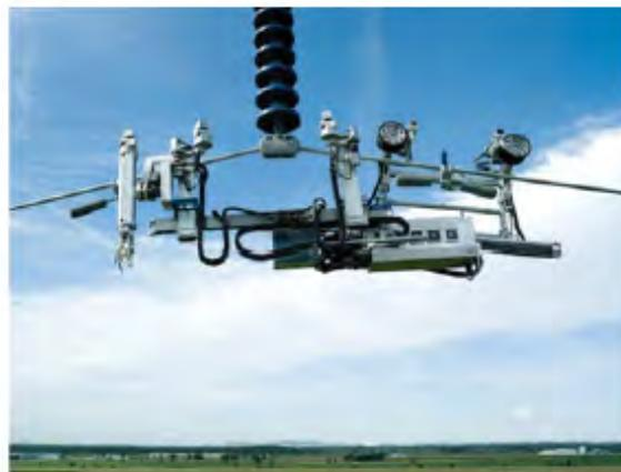
FIGURE 2.2: The LineScout robot on a transmission line [46].
