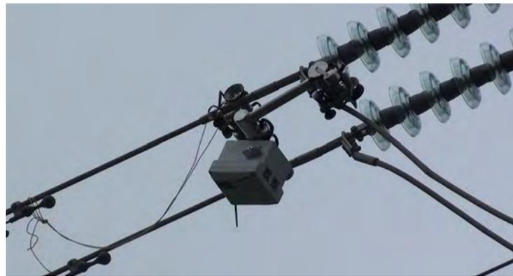
(B) PLIR on a transmission line test in New Zealand.
