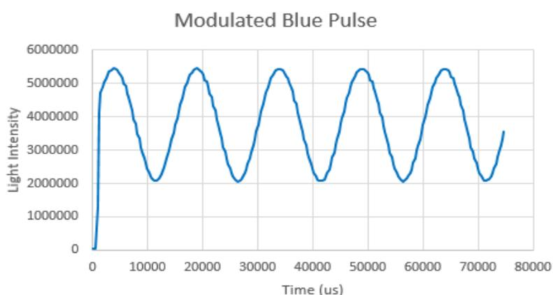
*Figure 31: Modulated excitation light pulse.*
