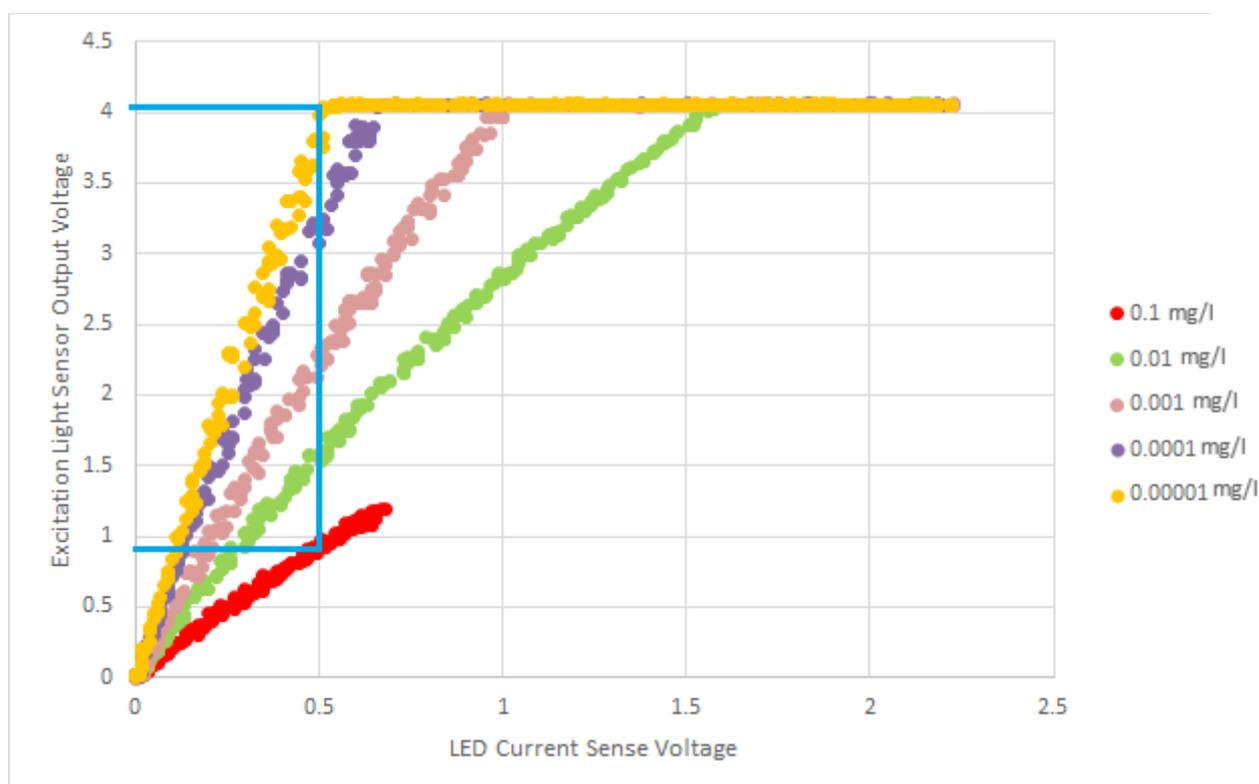
Figure 45: Excitation light changes for concentration and current.
