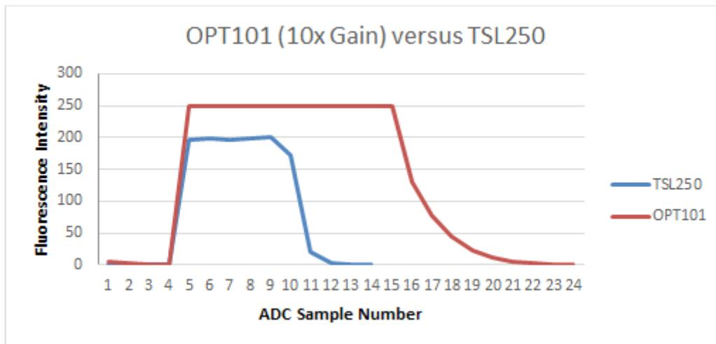
Figure 18: OPT101 (10x gain) delay versus TSL250.
