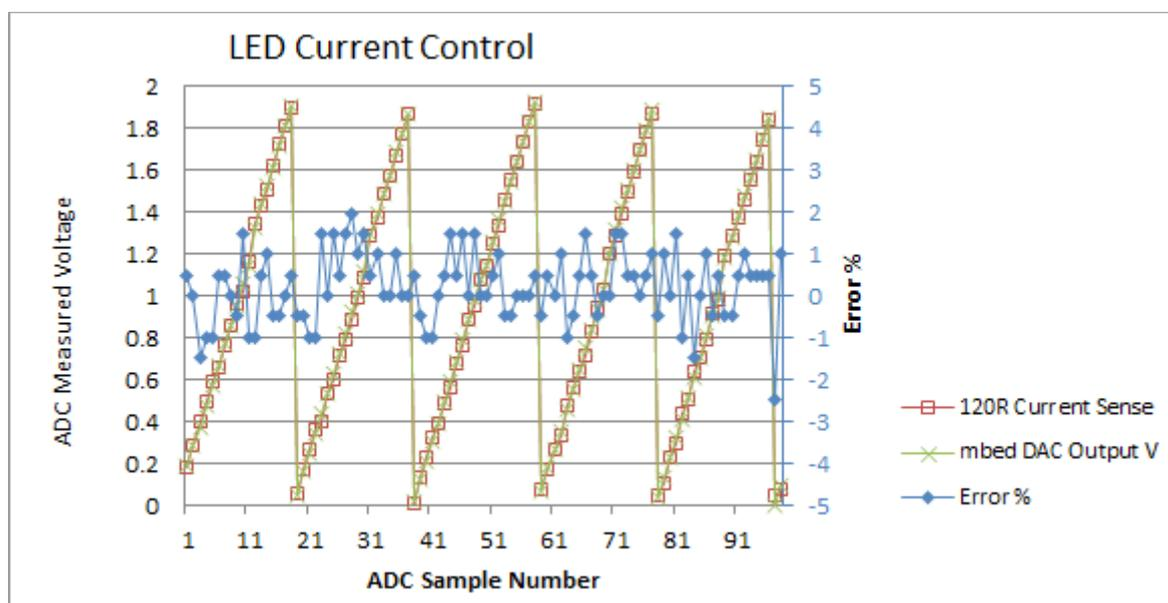
Figure 28: Current control accuracy
