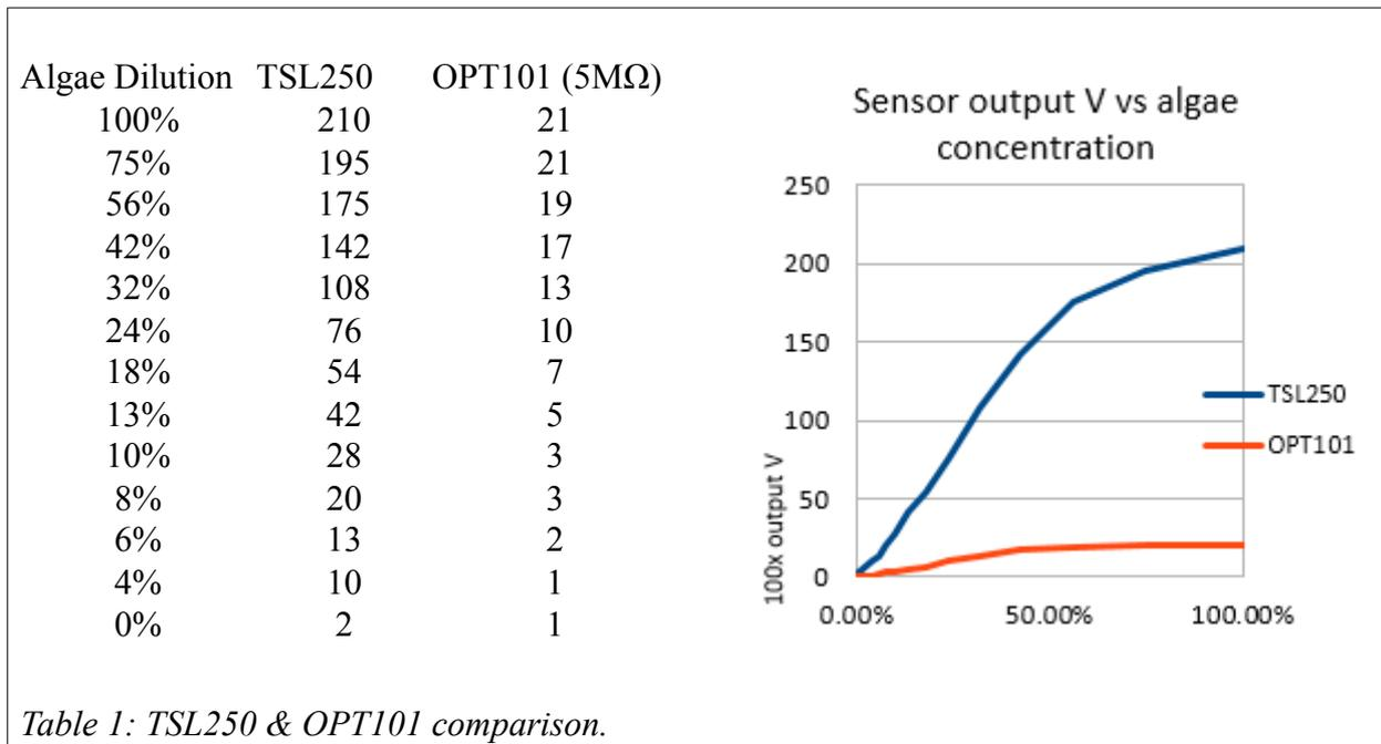
With its standard gain the OPT101 sensor provided very low output voltages (< 0.4 V) even for high algae concentrations. When the OPT101 gain was increased to 5 and 10 times the normal
