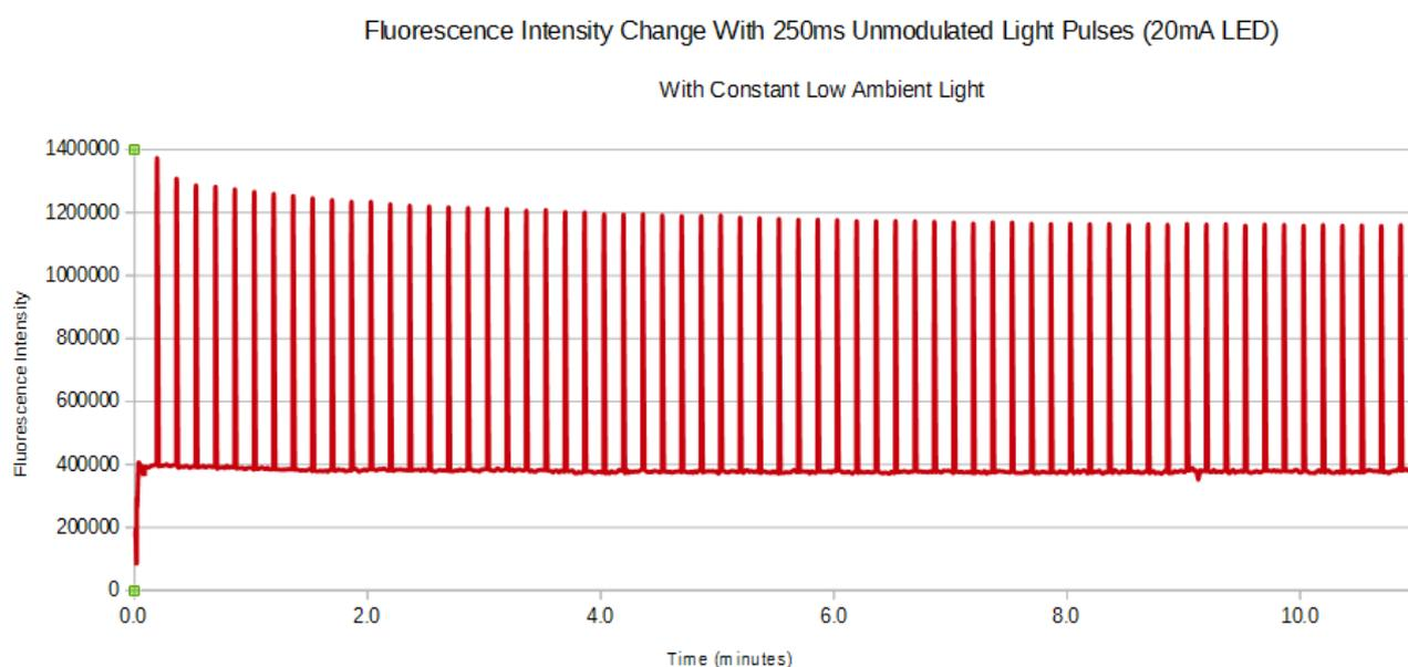
Figure 35: Fluorescence change with unmodulated 250 ms pulses.
