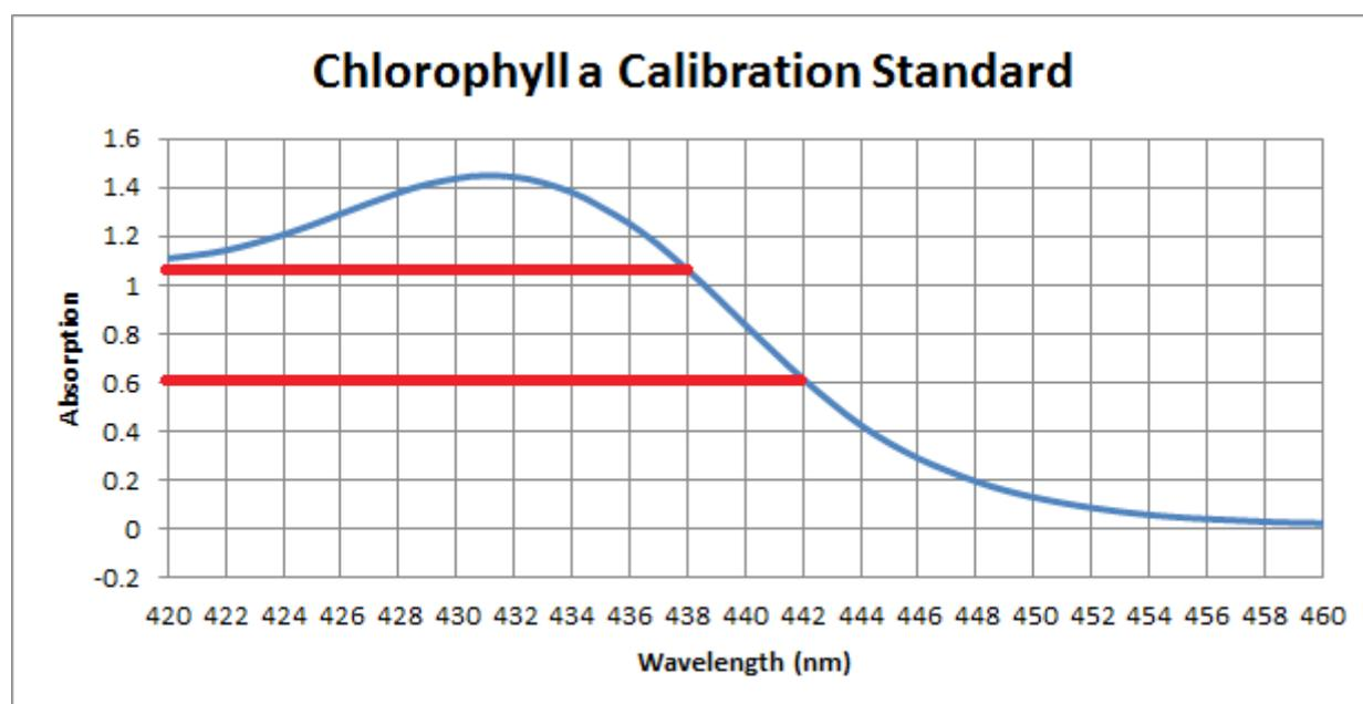
Figure 16: Effect of LED wavelength shift.
