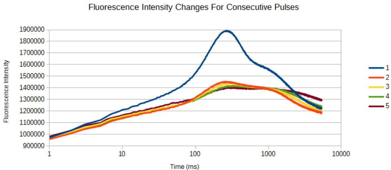
Figure 36: Fluorescence intensity change for consecutive pulses.
