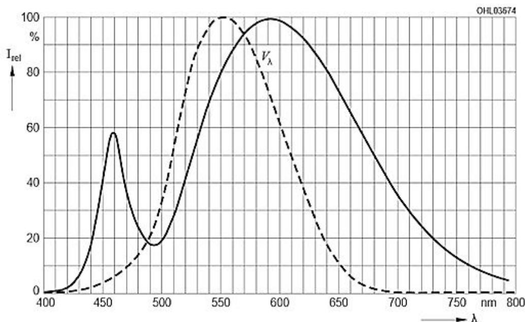
Figure 10: White LED emission spectrum.
