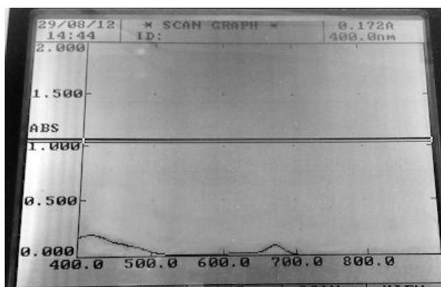
Figure 42: Spinach extracted chlorophyll absorbance spectrum.
