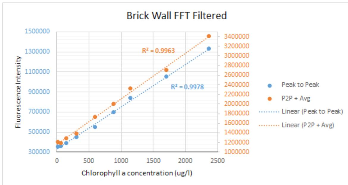
Figure 51: "Brick wall" FFT filtered fluorescence relationship to concentration.
