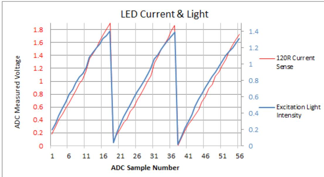
Figure 13: LED current vs LED light intensity.
