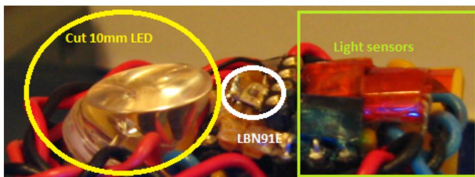
Figure 12: Cut LED & SMD LED layout.
