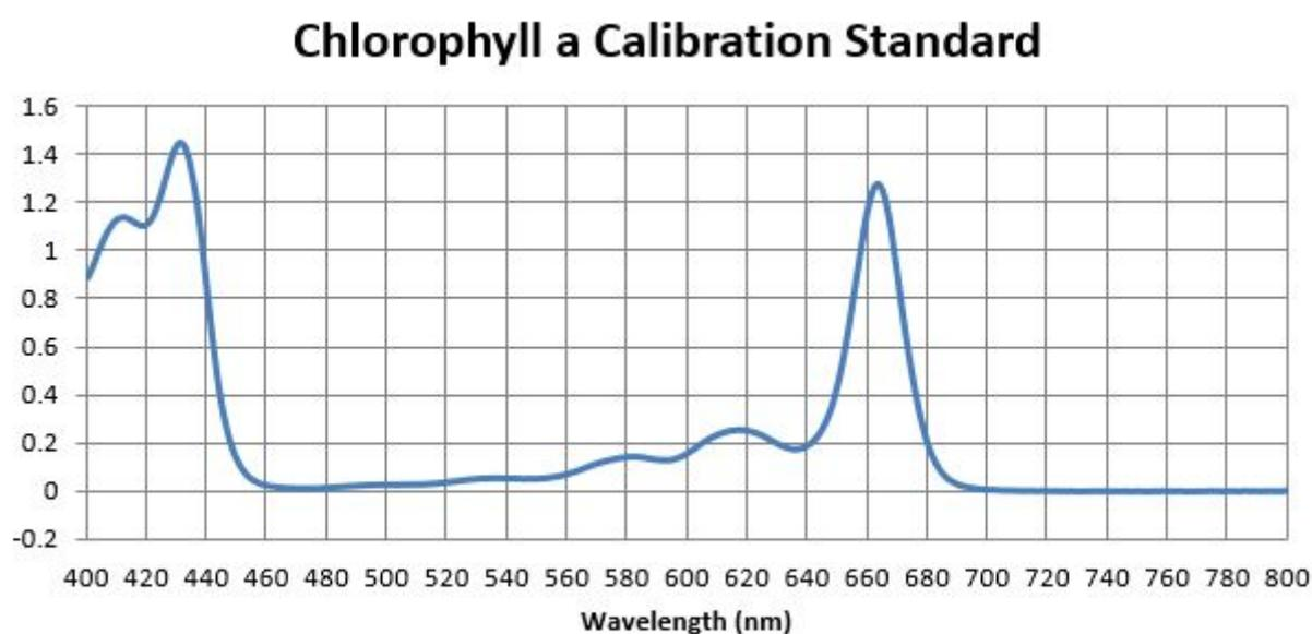
Figure 46: Absorption spectrum of calibration standard.
