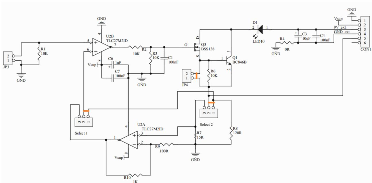
Figure 27: LED current control circuit.
