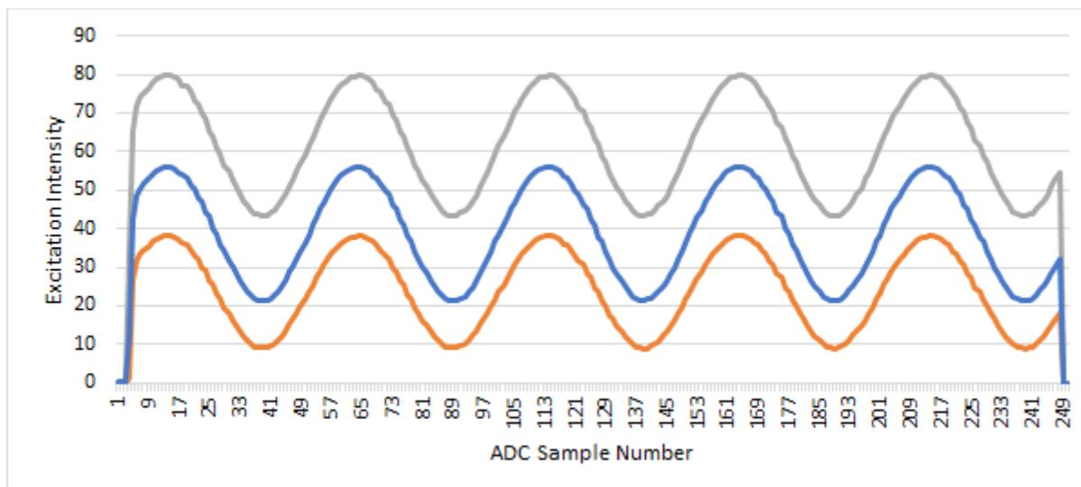
Figure 17: Modulated light pulses with different DC offsets.
