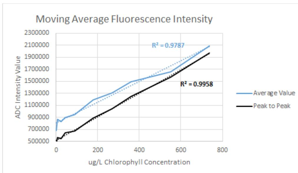
Figure 48: Moving average fluorescence vs chlorophyll concentration.
