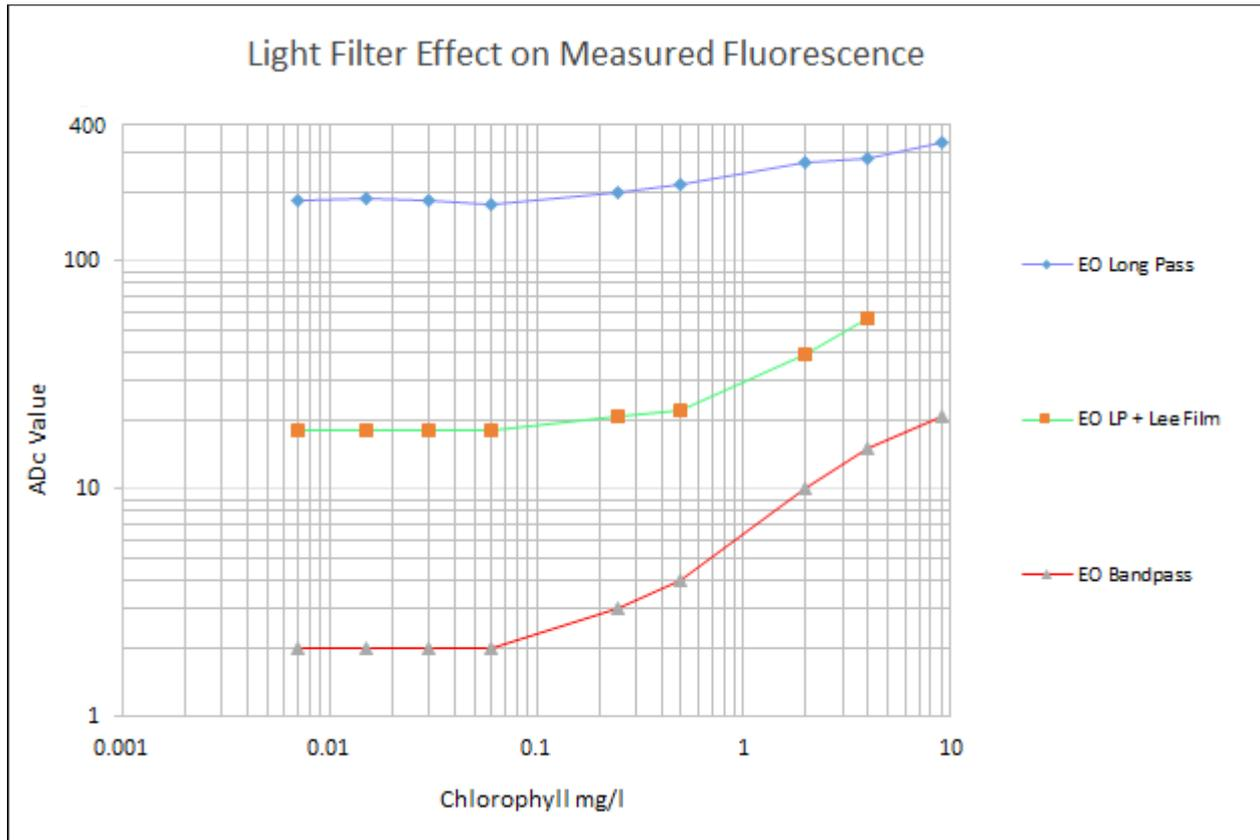
Figure 20: Effect of different filters on measured fluorescence.
