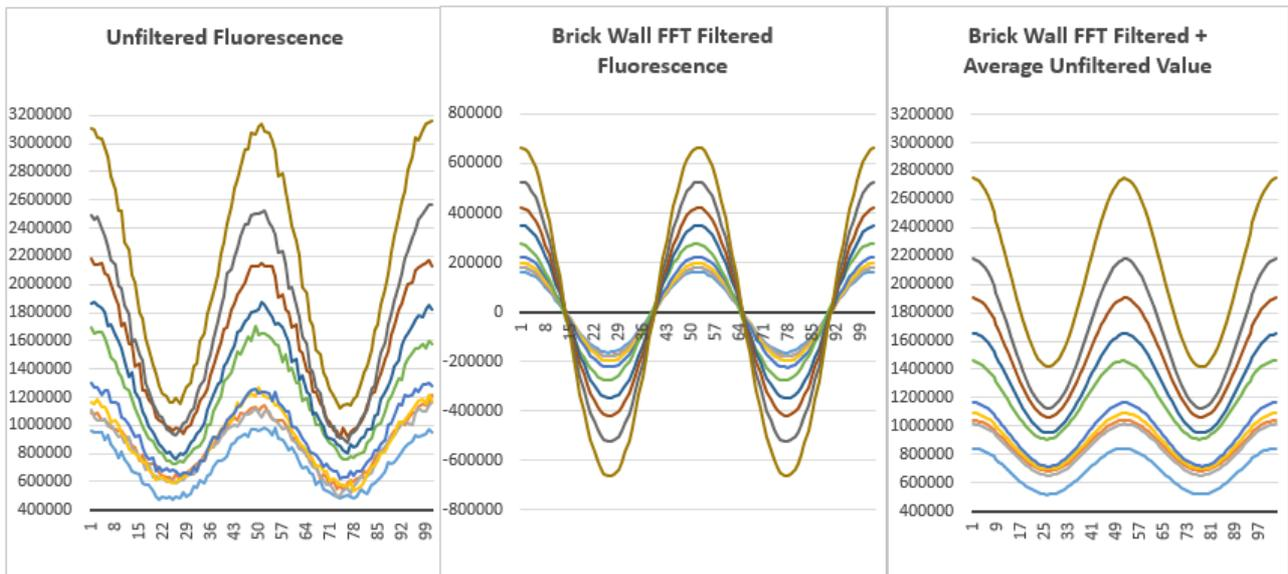
Figure 50: FFT “brick wall” filtered signals & unfiltered signals.
