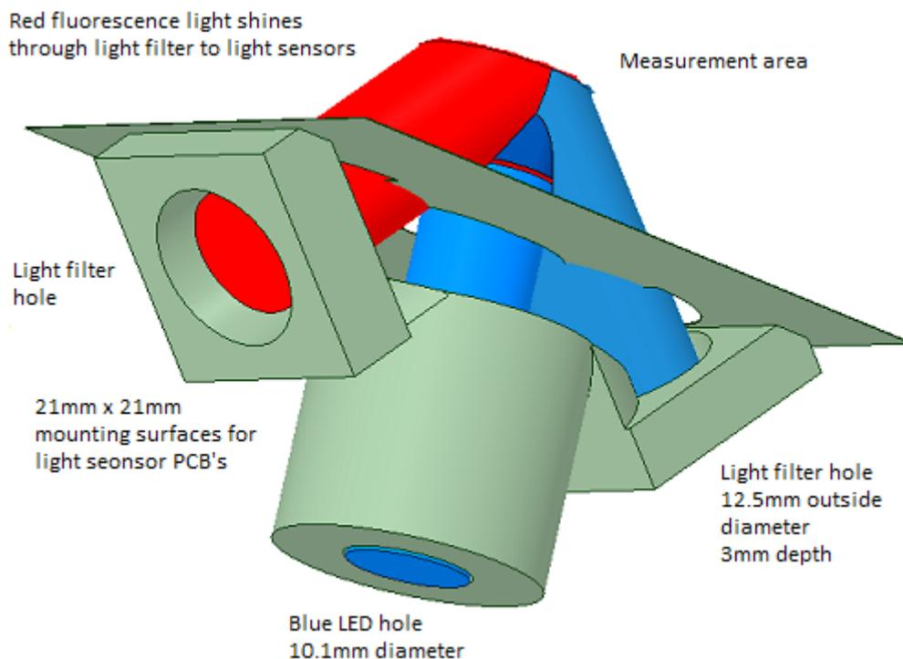
Figure 55: Flat faced FICC prototype light sensor locations.
