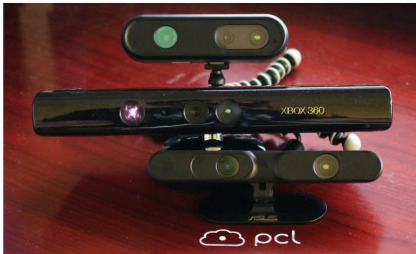
Figure 2.4: Most popular depth cameras used in research (from top to bottom: the Primesense reference design, Microsoft Kinect and Asus Xtion Pro) taken from [22].
