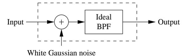
The Shannon-Hartley theorem states that the channel capacity is given by
